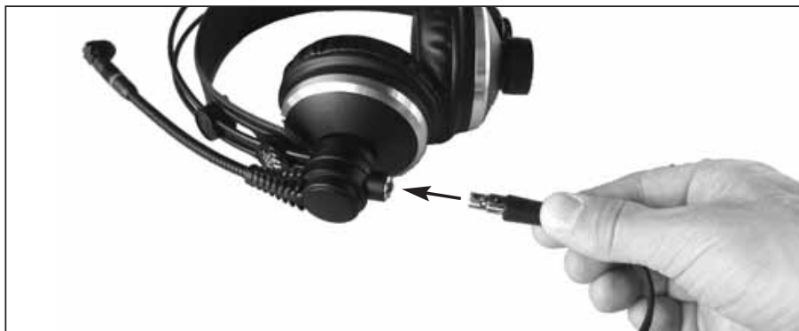
Fig. 1: Plugging the connecting cable into the headset.
