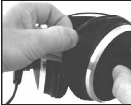
Fig. 6: Replacing ear pads.
