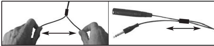
Fig. 2: Separating microphone and headphone cables.
